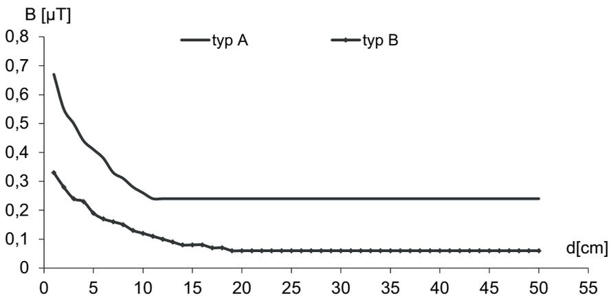
Fig. 2. Characteristics of avoiding the B magnetic field induction [ $\mu\text{T}$ ] within the distance function d[cm] for a stereo system, in the ELF frequency range
