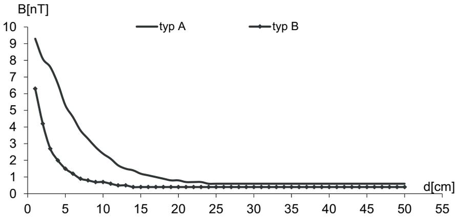
Fig. 3. Characteristics of avoiding the B magnetic field induction [nT] within the distance function  $d$ [cm] for a stereo system, in the VLF frequency range
