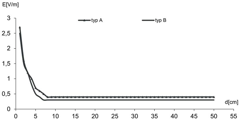
Fig. 4. Characteristics of avoiding the E electric field strength [V/m] within the distance function  $d$ [cm] for a stereo system, in the VLF frequency range
